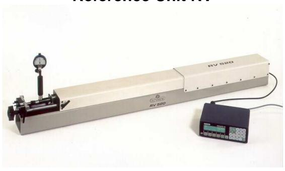
Comparison measuring instruments can only be as precise as the reference standard necessary for calibration purposes.
